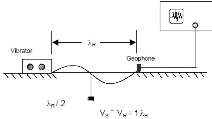
Figure 2 Steady-State Surface Wave Test
