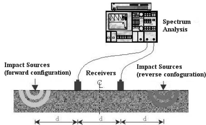
Figure 3 Spectral Analysis of Surface Wave
