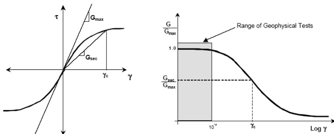
Figure1 Stress-strain curve with variation of shear modulus and modulus reduction curve
